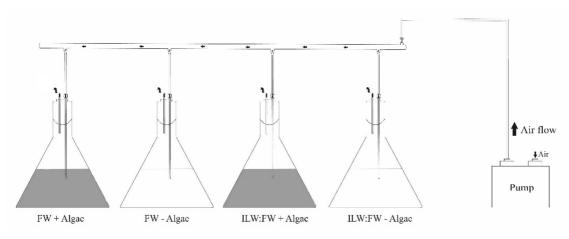
Figure 1. A schematic figure of the treatments at the laboratory-scale experiments for nutrient removal using filamentous algae *Cladophora*.
