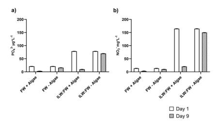
**Figure 3.** (a) initial and final (after 9 days of cultivation) concentration of phosphate in filtered water (FW) with (+) and without (-) *Cladophora* sp. and agricultural liquid waste (ILW:FW) at 25:75 ratio with (+) and without (-) *Cladophora* sp (b) initial and final (after 9 days of cultivation) concentration of nitrate in filtered water (FW) with and without *Cladophora* sp. and agricultural liquid waste (ILW:FW) at 25:75 ratio with (+) and without (-) *Cladophora* sp.
